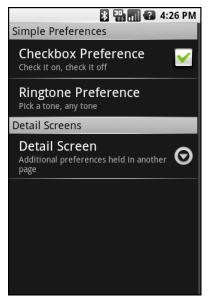
Figure 21–4. The Structured project's preference UI, showing categories and a screen placeholder
